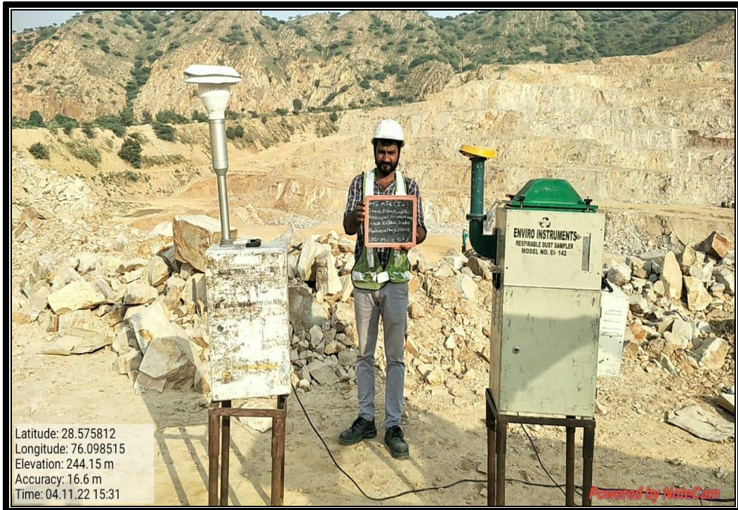
Ambient Air Quality Monitoring
