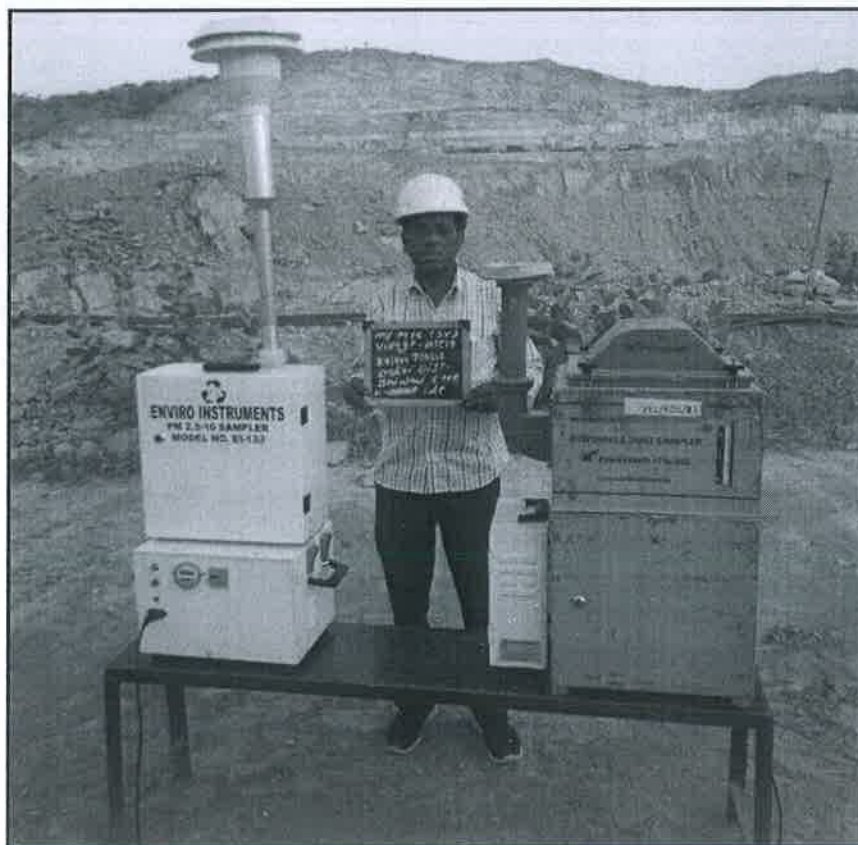
Ambient Air Quality Monitoring
